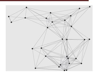
Fig.3.2.1. The original topology: A MANET with 30 nodes randomly deployed in 800 x 800 m<sup>2</sup>area
