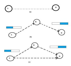
Fig.2.1.1. Three transmission protocols: a) direct transmission via a point to point conventional link. b) Multi – hop transmission via a two- hop manner occupying two time slots. c) Cooperative transmission via a cooperative diversity occupying two
